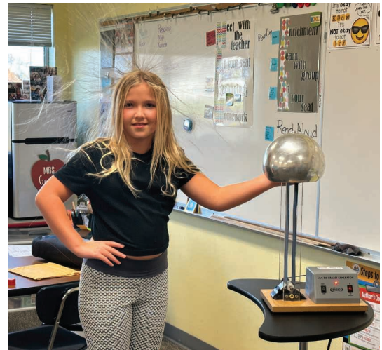
A Van de Graaff generator demonstrated the movement of electrons with some hair-raising and shocking results for a student.
