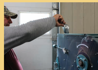
The seeds are fed into a hammer mill to break apart remaining plant material from the seeds.
