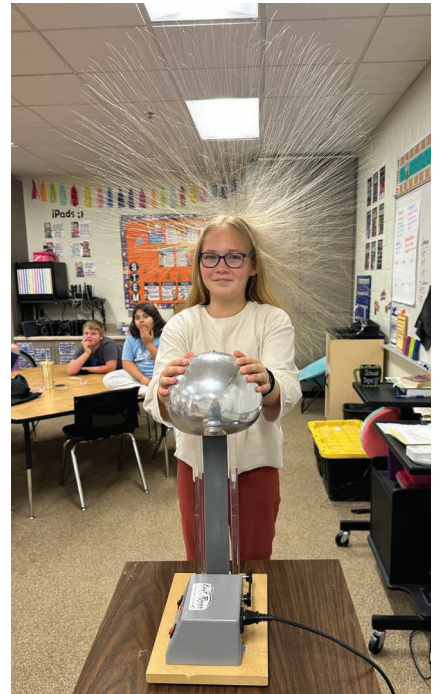
A Van de Graaff generator demonstrated the movement of electrons with some hair-raising and shocking results for a student.
